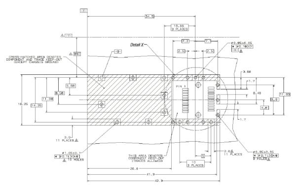
Detum and Basic Dimension Established by Customer Rads and Vias are Chassis Ground, 11 Places Through Holes are Unplated
