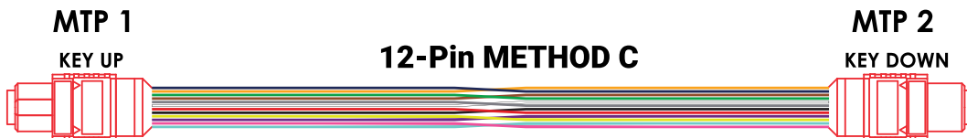
MTP-12 Connector Fiber Assignments
