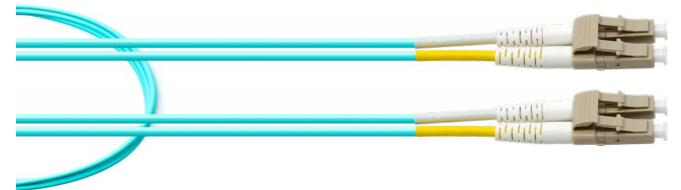
The GigaTech Products GT-LCLCDM4A-xM fiber optic patch cords are ideal for short distance patching applications. These fiber optic cables have been built to exceed industry standards and are tested for insertion loss and reflectance on all connectors. They are constructed using Corning glass within UL certified OFNR (Riser) rated jacket with Kevlar yarn, and are factory terminated resulting in uncompromised performance.
