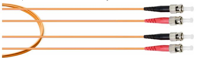
The GigaTech Products GT-STSTDM20-xM fiber optic patch cords are ideal for short distance patching applications. These fiber optic cables have been built to exceed industry standards and are tested for insertion loss and reflectance on all connectors. They are constructed using Corning glass within UL certified OFNR (Riser) rated jacket with Kevlar yarn, and are factory terminated resulting in uncompromised performance.
