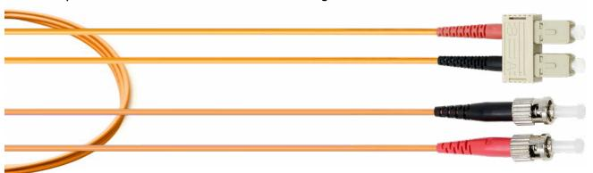
The GigaTech Products **GT-SCSTDM10-xM** fiber optic patch cords are ideal for short distance patching applications. These fiber optic cables have been built to exceed industry standards and are tested for insertion loss and reflectance on all connectors. They are constructed using Corning glass within UL certified OFNR (Riser) rated jacket with Kevlar yarn, and are factory terminated resulting in uncompromised performance.
