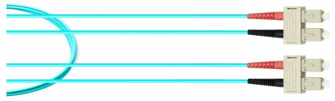
The GigaTech Products GT-SCSCDM4A-xM fiber optic patch cords are ideal for short distance patching applications. These fiber optic cables have been built to exceed industry standards and are tested for insertion loss and reflectance on all connectors. They are constructed using Corning glass within UL certified OFNR (Riser) rated jacket with Kevlar yarn, and are factory terminated resulting in uncompromised performance.
