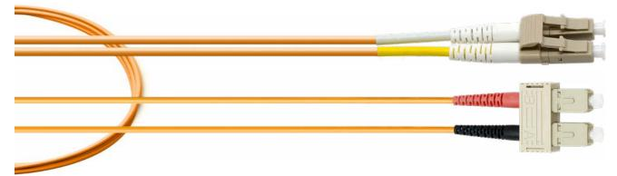
The GigaTech Products **GT-LCSCDM20-xM** fiber optic patch cords are ideal for short distance patching applications. These fiber optic cables have been built to exceed industry standards and are tested for insertion loss and reflectance on all connectors. They are constructed using Corning glass within UL certified OFNR (Riser) rated jacket with Kevlar yarn, and are factory terminated resulting in uncompromised performance.
