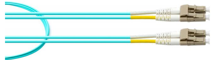
The GigaTech Products GT-LCLCDM3A-xM fiber optic patch cords are ideal for short distance patching applications. These fiber optic cables have been built to exceed industry standards and are tested for insertion loss and reflectance on all connectors. They are constructed using Corning glass within UL certified OFNR (Riser) rated jacket with Kevlar yarn, and are factory terminated resulting in uncompromised performance.
