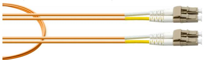
The GigaTech Products **GT-LCLCDM20-xM** fiber optic patch cords are ideal for short distance patching applications. These fiber optic cables have been built to exceed industry standards and are tested for insertion loss and reflectance on all connectors. They are constructed using Corning glass within UL certified OFNR (Riser) rated jacket with Kevlar yarn, and are factory terminated resulting in uncompromised performance.
